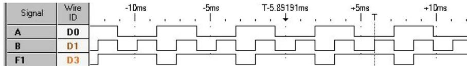
Figure 5.5 Waveforms of the logic analyser while investigating F1.
