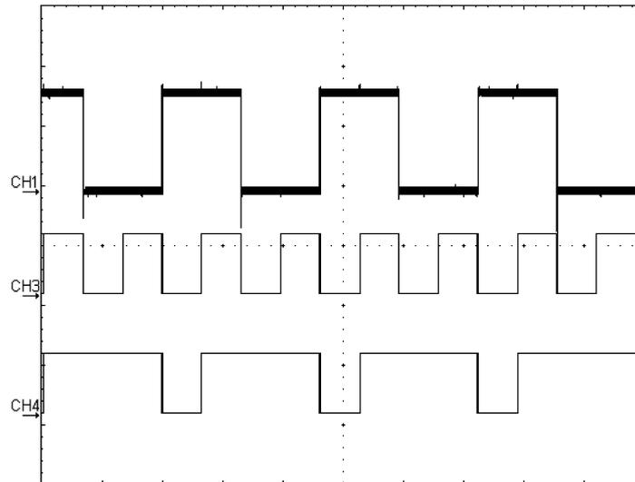
**Figure 5.3** Oscilloscope image, investigating F1 (CH1 - A, CH3 - B, CH4 - F1).
