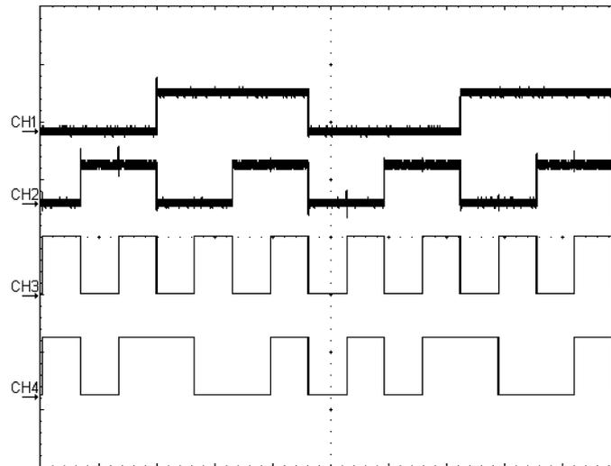
**Figure 5.4** Oscilloscope image, investigation of F2 (CH1 - A, CH2 - B, CH3 - C, CH4 - F2).
