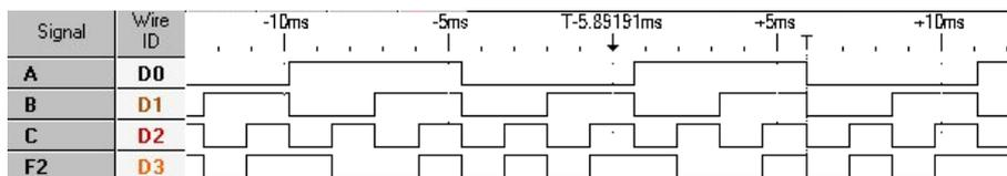
Figure 5.6 Waveforms of the logic analyser while investigating F2.
