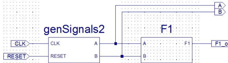
**Figure 5.2** Analysed combinatorial circuit, connected to the counter-based stimulus generator (**F1test.sch**).
